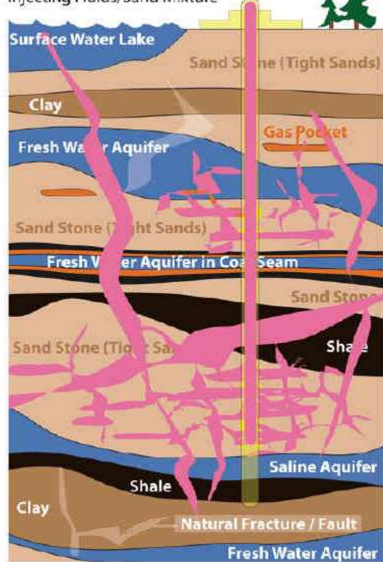
Hydraulic Fracing Diagram 4 Injecting Fluids/Sand Mixture
